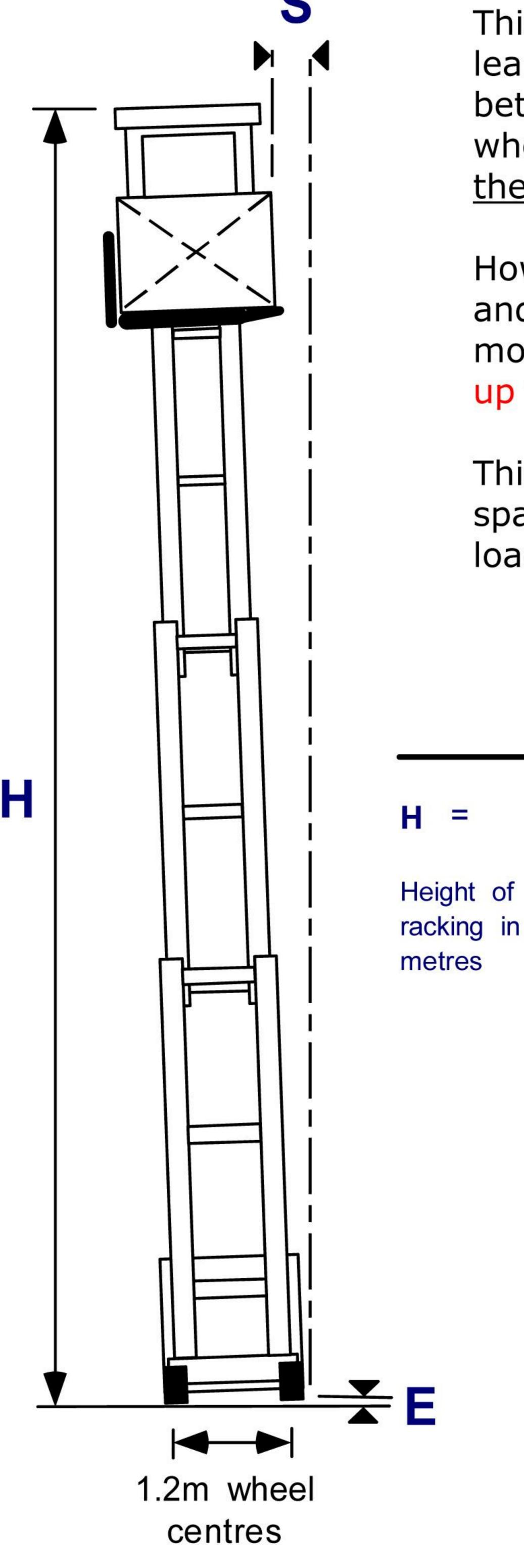
This table shows the relationship between the static lean of a forklift truck, due to the difference in elevation between the left and right hand forklift truck load wheels, and the height of the racking, <u>assuming that</u> the mast is a rigid structure.
